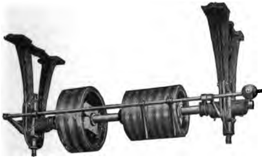
FIG. 145.—Countershaft with Fast and Loose Pulley on Right. A shifting rod throws the belting from one pulley to the other.
